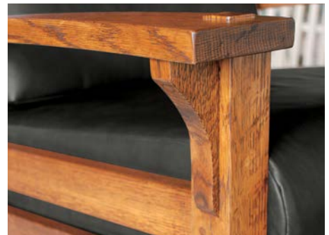
Detail of arm corbels
